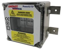
To complement our FSP offering, we provide a range of Terminal Boxes for incoming and outgoing power cables into new or legacy equipment. These boxes can terminate 2 or 4 core cables and have the ability to output 2 or 4 cores of cable to allow ultimate flexibility to the end user. These are available with stud or tunnel terminals with boxes accommodating cables from 6-50mm<sup>2</sup>, 16-120mm<sup>2</sup> or 6-185mm<sup>2</sup> (stud only).
